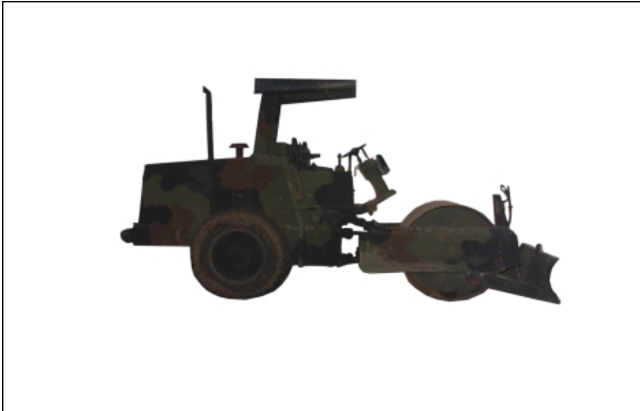
Figure 13-1. Vibratory compactor (Model CS-433C)
